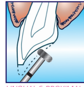
LINGUAL & PROXIMAL REDUCTION: Provides fast bulk reduction of lingual and proximal surface.
